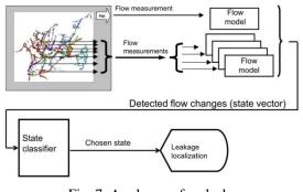
Fig. 7. A scheme of an leakage location method [30]
